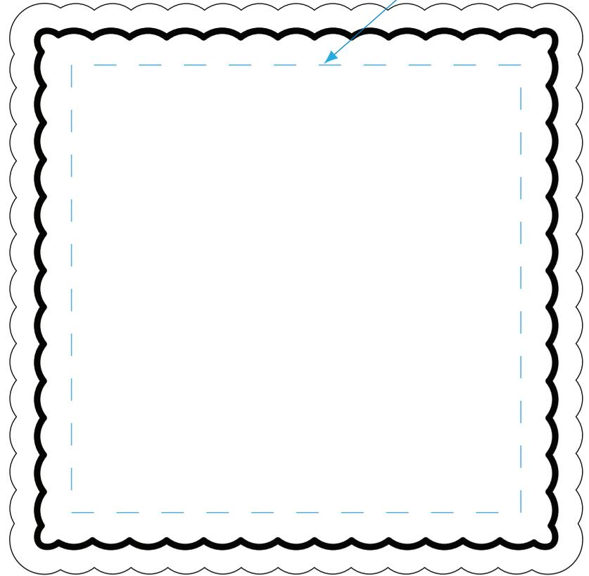
**The registration movement is 2 to 3 mm per color in any direction
