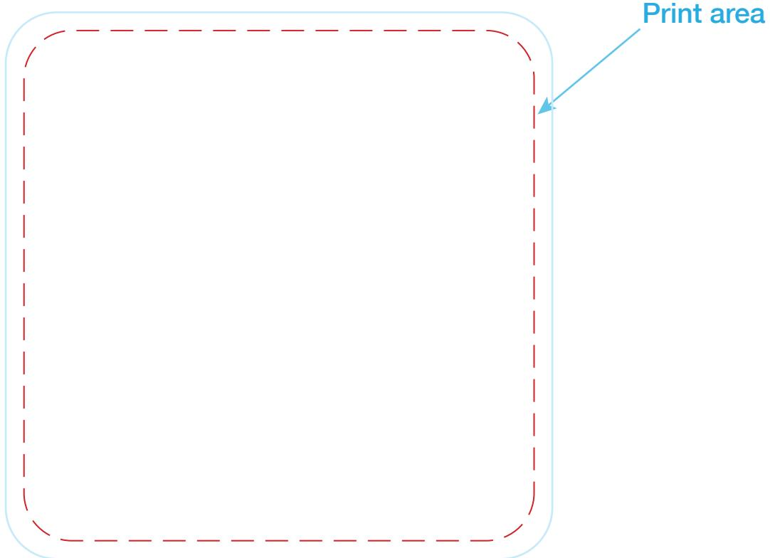
The registration movement is 2 to 3 mm per color in any direction
