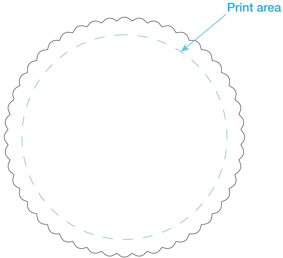
The registration movement is 2 to 3 mm per color in any direction
